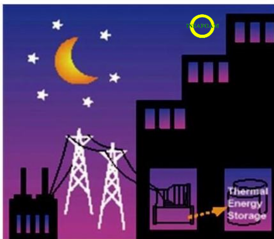
Energy generated by the utilities more efficiently at night, is used to make ice.
